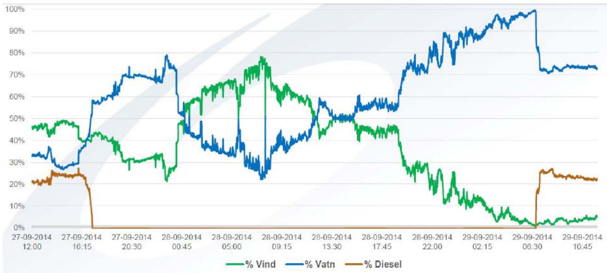
Figure 11-4: Balanced grid operation for two days in September 2014. The wind generation is mainly balanced by hydro power in this specific period, but hydro is limited so the diesel generation is also utilized.
