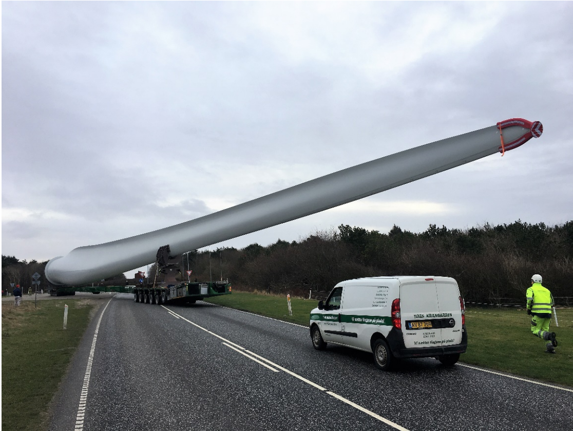
Figure 7. Transport of blade. Photo: Lasse Dieckmann
