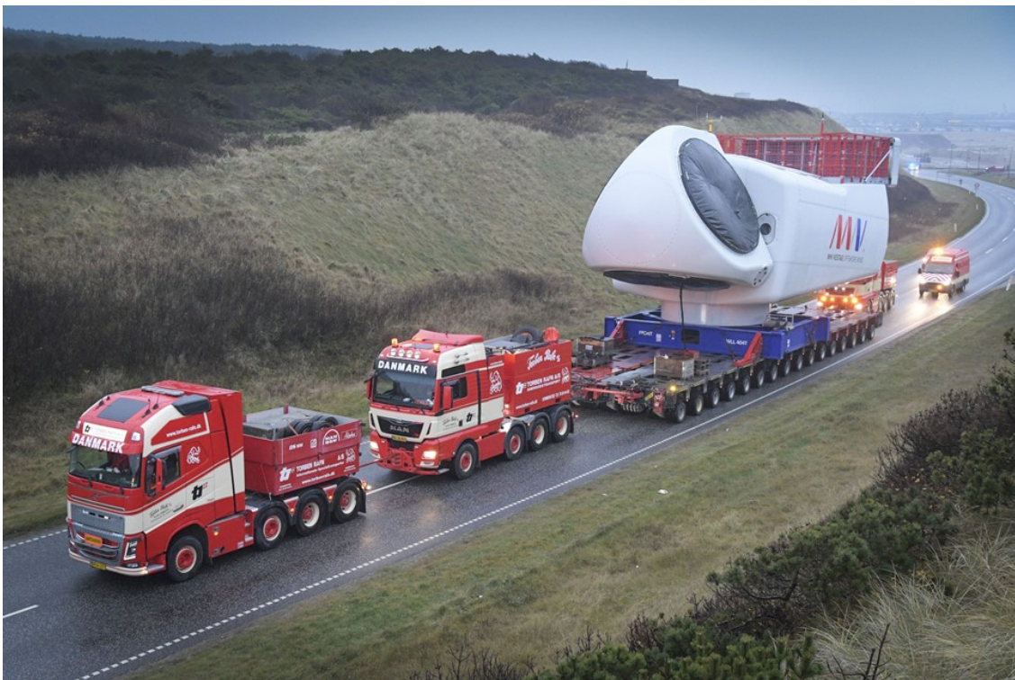
Figure 6. Transport of nacelle from Hanstholm to Østerild, November 2019. Photo: Peter Mørk, Nordjyske
