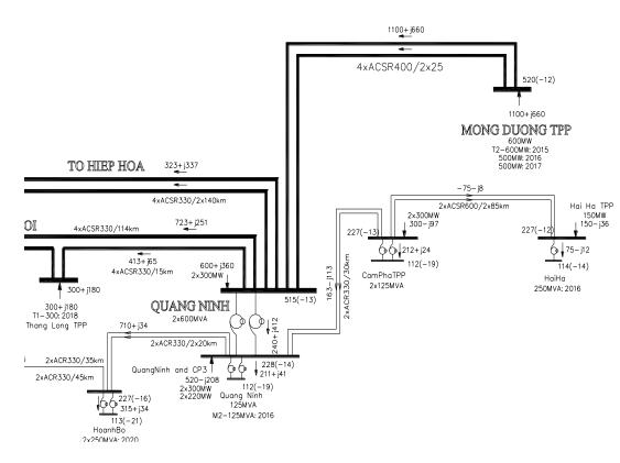
Figure 6: The 500kV and 220kV power grid of Quang Ninh province in year 2020.
