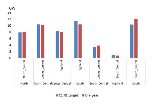
Figure 85: Comparing Transmission capacity between regions in 2050 in the Dry year and C1 RE target scenarios.
