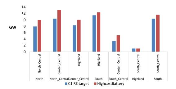
Figure 76: Comparing Transmission capacity between regions in 2050 of the High cost Battery and C1 RE target scenarios.
