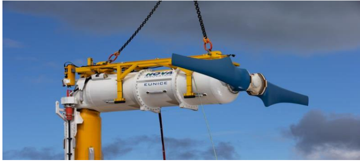
Figure 48: 500 kW direct drive turbine [16]
