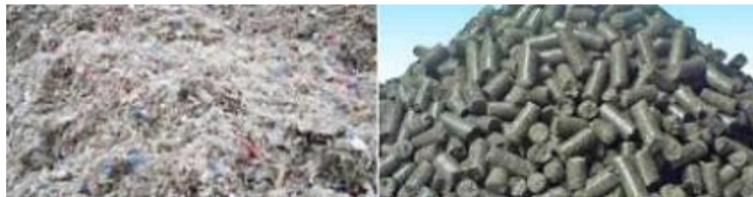
RDF fluff (left) and RDF pellets (right) (Source: MEMR (2020), Waste to Energy Guidebook)
