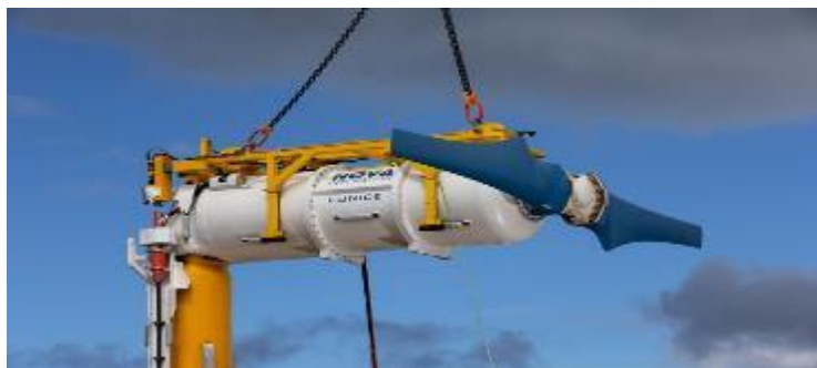
500 kW direct drive turbine (ref. 19)
