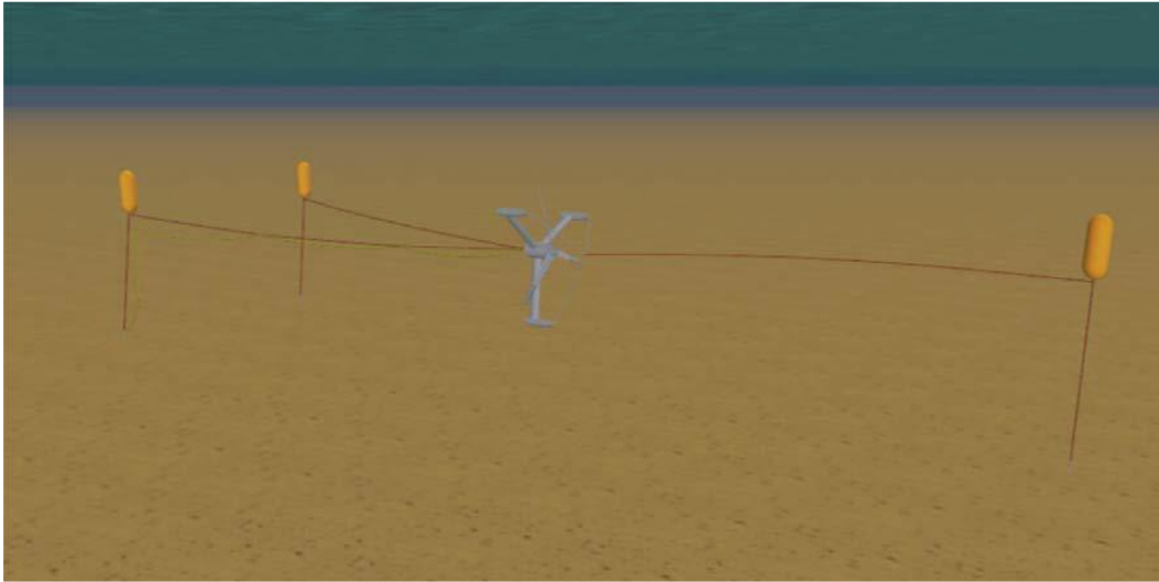
Foundation types: Second generation devices - Mooring system based on wires and buoys. (ref. 7)
