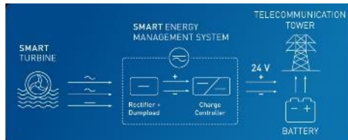
Pico hydropower with hydrokinetic turbine for remote telecommunication towers (ref. 17)
