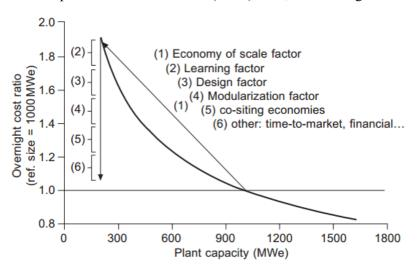
(Ref. 12 and ref. 13) considers four plant sizes (1600 MWe, 1200 MWe, 300 MWe, 150 MWe) to compare the "economy of scale" and the "economy of multiples" paradigms and two scenarios: NPPs deployed by a big utility and two minors and NPPs deployed by a single utility. The main results are:
