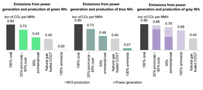
Figure 10. Emission reduction potential depending on the ammonia source [Ref.2]
