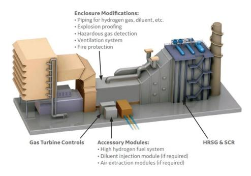
Figure 19: Example of a hydrogen gas turbine and its components
