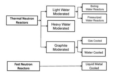
Figure 95: Classification of nuclear reactors
