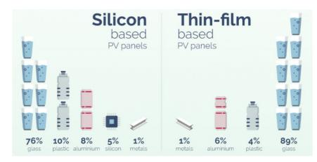
Figure 41: Main materials in a silicon based and thin film solar PV panel. (ref. 22)
