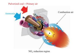
*Figure 8. Schematic diagram of the modified burner to co-firing ammonia [Ref.1]*
