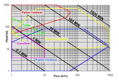
*Figure 32: Hydropower turbine application chart (ref. 2)*
