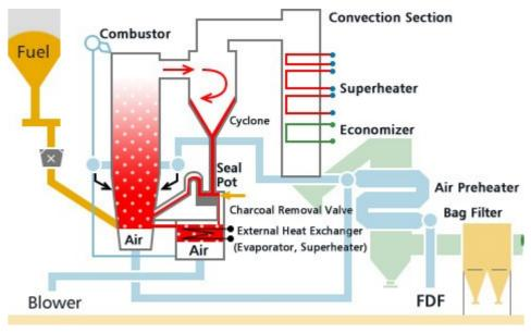
Figure 144: CFB boiler scheme (Ref. 2)
