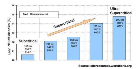
*Figure 2: Definitions of sub-, super-, and ultra-supercritical plant (ref. 6). The same definitions apply to Anthracite coal.*
