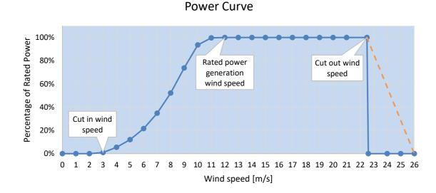
Figure 54: Power curve for a typical wind turbine (Ref. 48).
