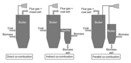
Figure 82: Different biomass co-firing configurations (ref. 15)
