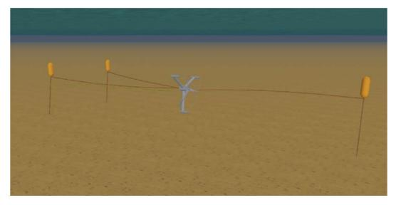
Figure 64: Foundation types: Second generation devices - Mooring system based on wires and buoys.[7]
