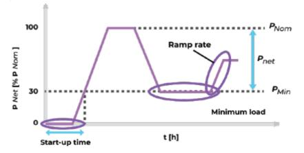
*Figure 3: Key flexibility parameters of a power plant [3].*
