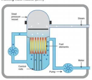
A Boiling Water Reactor (BWR)
