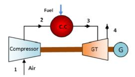
Figure 155: Process diagram of a Simple-Cycle Gas Turbine (SCGT) (ref. 1)
