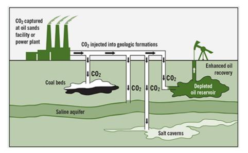
Figure 23. Post-capture treatment of CO<sub>2</sub>. Source: Energywatch.
