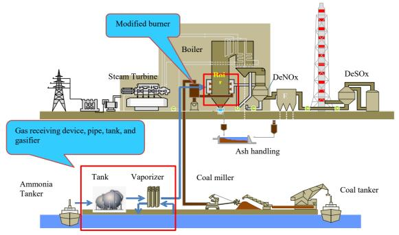
Figure 7. Facilities to be implemented and improved at a coal ammonia co-fired power plant
