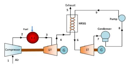
Figure 166: Process diagram of a CCGT (ref. 1)
