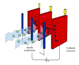
Figure 4: Principle behind electrostatic precipitator (ref.4).
