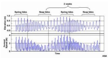
*Figure 57: Time series representation of spring and neap tide along with correlation with tidal current speed variation.[3]*
