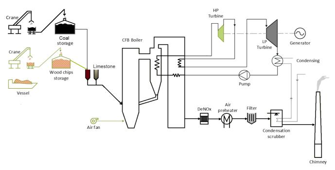
*Figure 13. Sketch of a CFB coal plant co-firing with wood chip. The green elements indicate the equipment that needs to be added, replaced or refurbished.*
