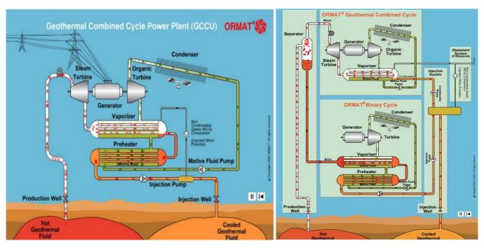
Figure 91: Hybrid/Combined Cycle plant (ref. 8)
