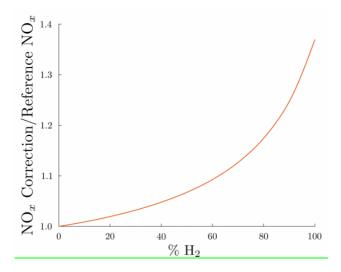
*Figure 21. Increase of NO<sub>x</sub> emission correspond to the H2 co-firing ratio according to [Ref. 9]*
