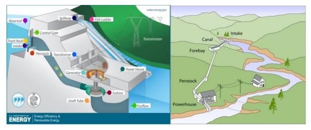
Figure 30: Reservoir and run-of-river hydropower plants (ref. 14)
