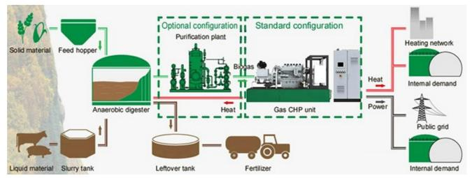
Figure 88: Biogas CHP working diagram (ref. 5).
