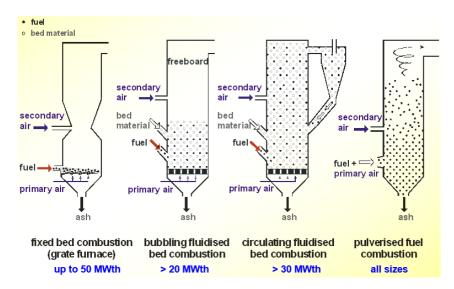
Figure 81: Technologies for industrial biomass combustion (ref. 4)
