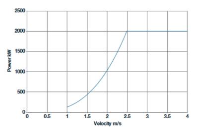
Figure 65: Sample power curve for tidal stream turbine.[9]
