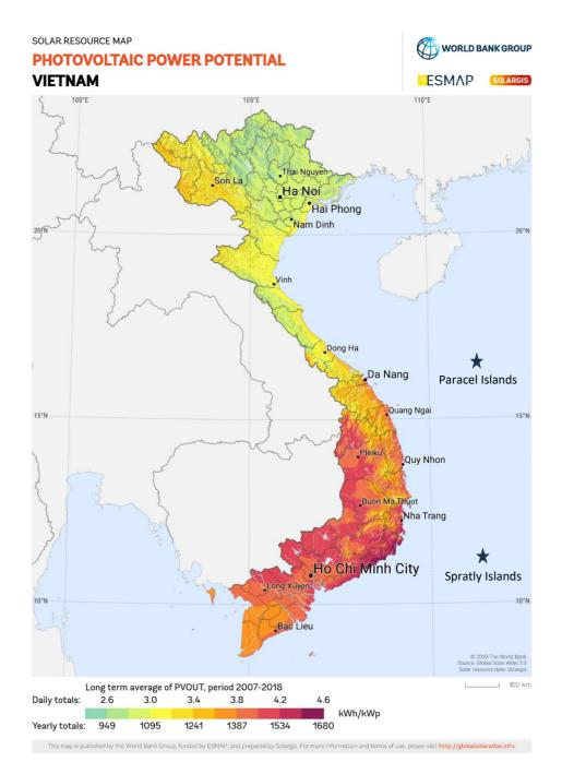
Figure 35: Full load hours (kWh/kWp) for PV in Viet Nam (Ref 7).
