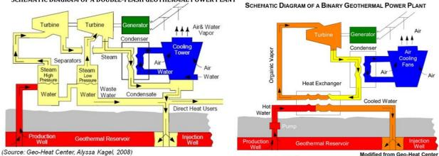
Figure 90: Double flashed (left) and binary (right) geothermal steam plants (ref. 7)
