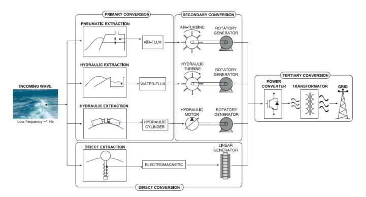
*Figure 73: Wave energy conversion stages [3]*
