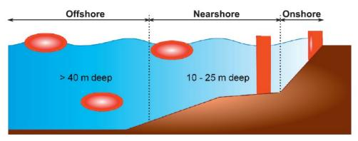
Figure 72: Location of wave energy converters [3]
