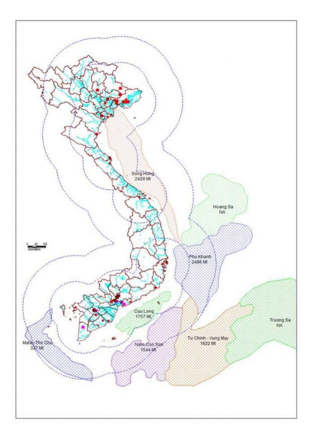
Figure 26: CO<sub>2</sub> storage potential in saline aquifers (150km and 300km circle around emission sources). The Paracel and Spratly Islands of Viet Nam are not shown in the map (Ref. 6, 20)
