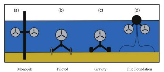
*Figure 63: Foundation types: First generation devices [7]*
