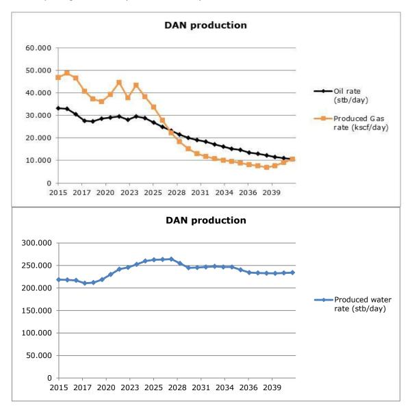
Figure 3-8 Maximum total expected production of oil, gas and water from the DAN project. Oil and water rate are provided as standard barrels per day, while the gas rate is provided as 1000 standard cubic feet of gas per day. The production forecast also accounts for the development projects.
