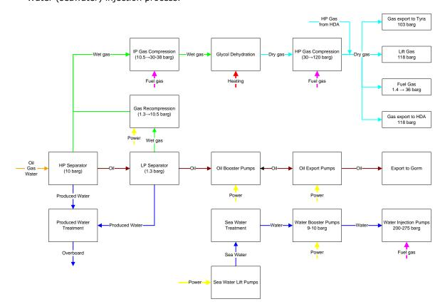
Figure 3-6 Simplified diagram of the process at Dan F
