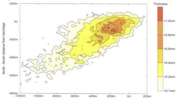
Figure 6-1 Sedimentation of discharged water based drilling mud modelled for a typical well /1/.
