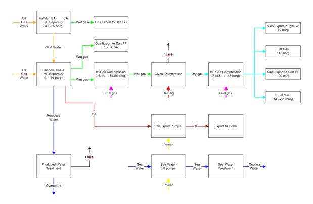
Figure 3-5 Simplified diagram of the process for the HALFDAN facilities.
