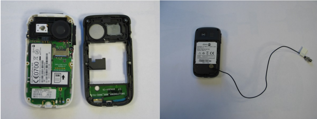
Pictures showing the Doro phone during conducted measurements. The phone is connected to the same base station emulator as used for the radiated measurements (a CMU200 from R&S serial number 110106).
