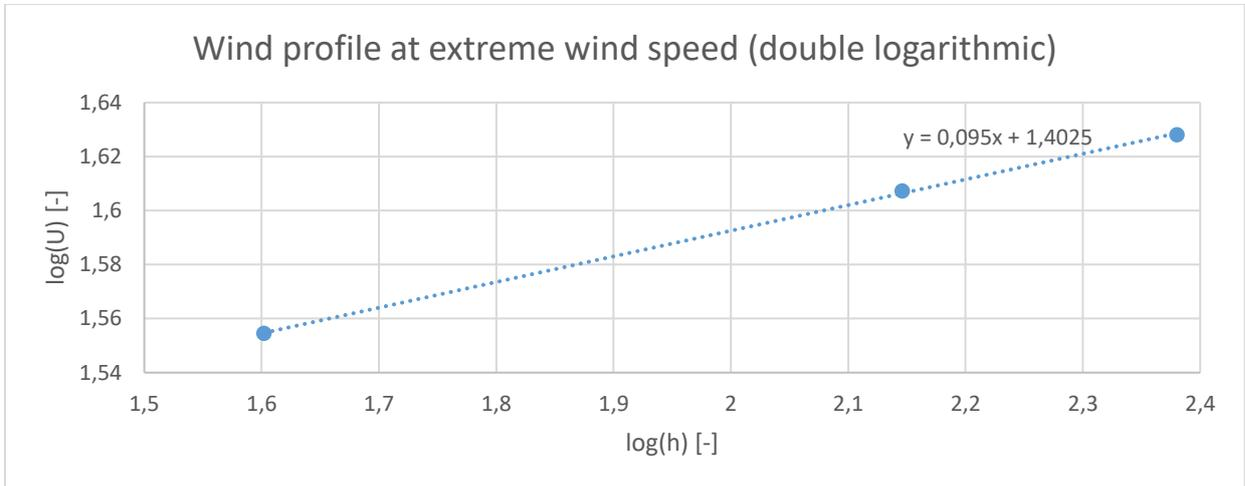
Figure 42. Fitted shear to extreme wind speed at three heights ASL.
