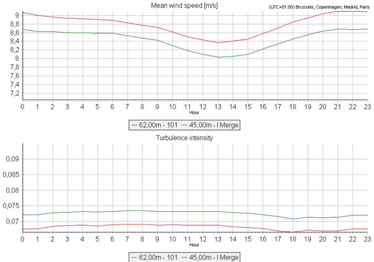
Figure 10. Daily variation of wind speed and turbulence intensity measured at Læsø met mast (62 and 45 m, 4 years)
