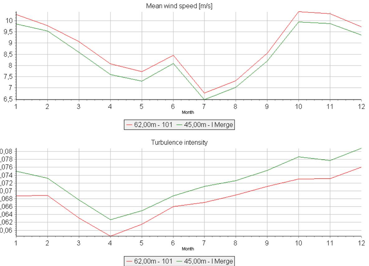
Figure 11. Monthly variation of wind speed and turbulence intensity measured at Læsø met mast (62 and 45 m, 4 years)
