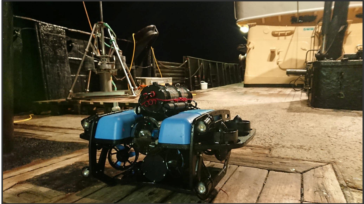
Figure 4-4 Remotely Operated underwater Vehicle (ROV) with integrated CTDO (on top) onboard the vessel "Cecilie".
