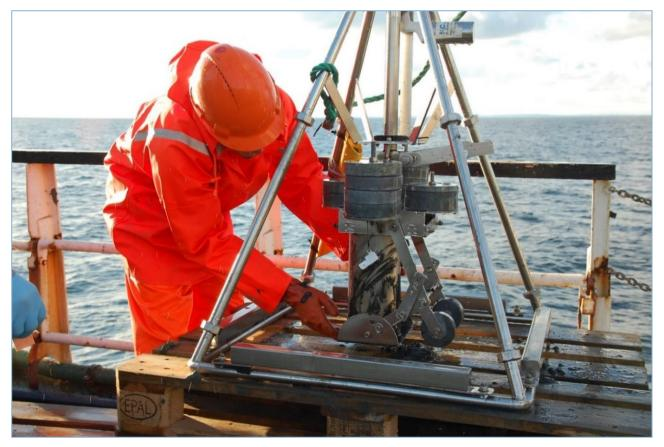
Figure 3-9. HAPS core sampler.
