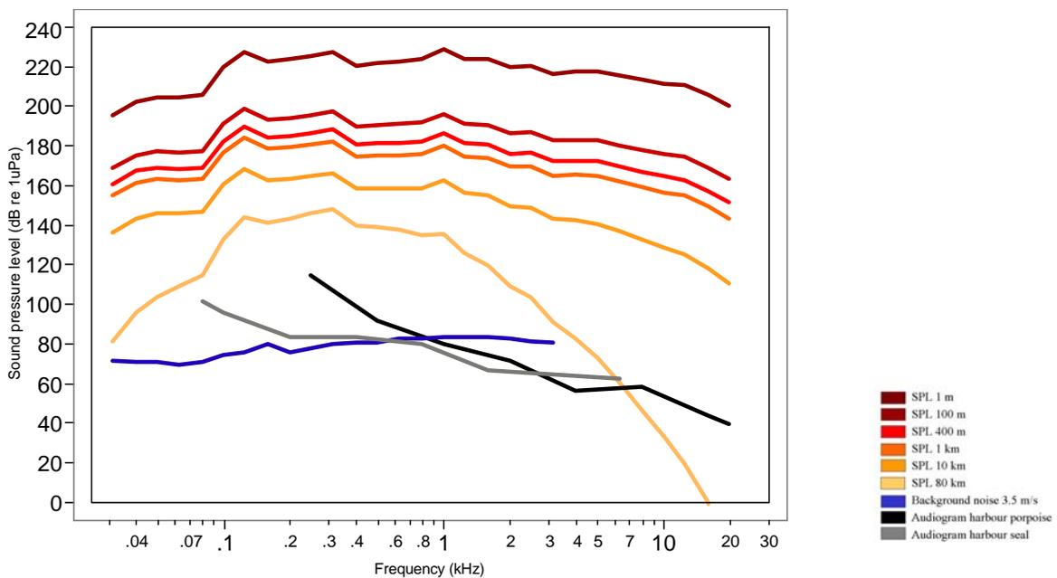
Figure 6.2. Pile-driving noise and background noise (see Figure. 6) compared to the audiogram of harbour porpoises and harbour seals (audiogram values as  $dB_{rms}$  re  $1 \mu Pa$ ; after Kastelein et al., 2002 and Kastak & Schusterman, 1998).
