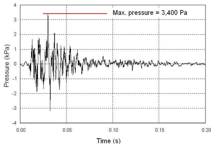
Figure 3.14. Waveform of an impact-pile pulse (after ITAP, 2005).
