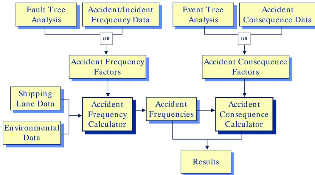
**Figure 13-1: Block Diagram of MARCS**
