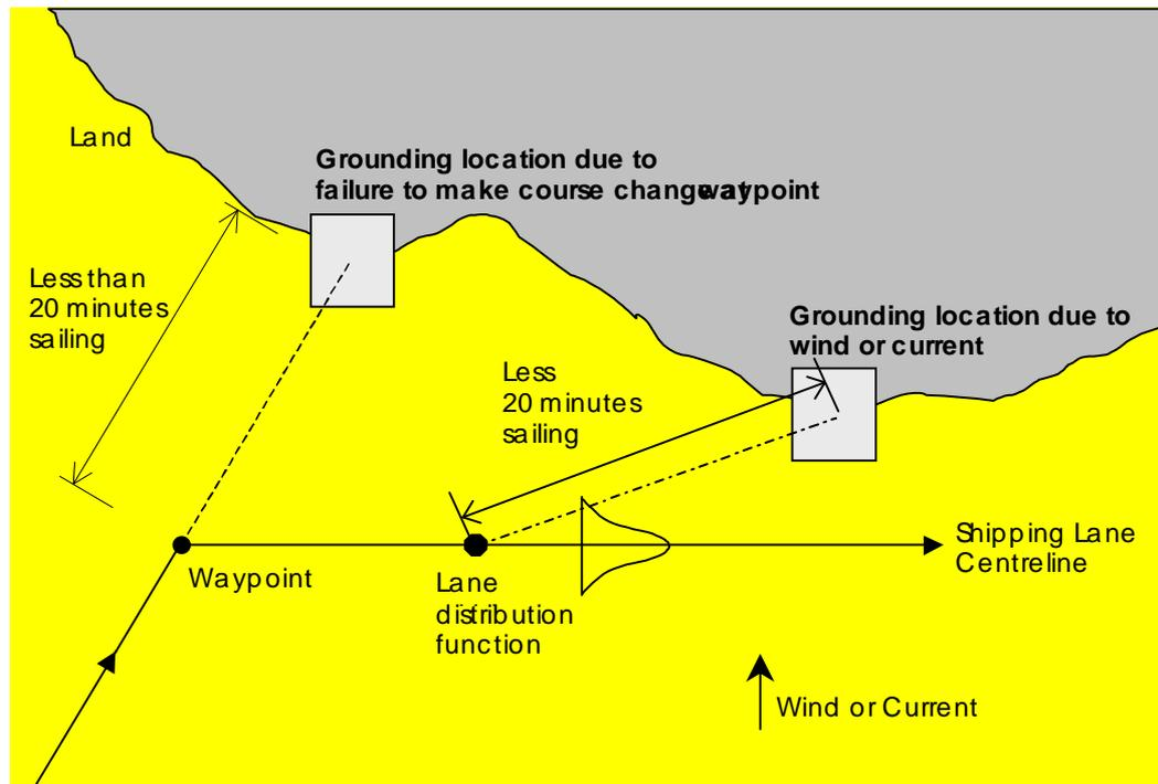
**Figure 13-5: Graphical representation of the powered grounding model**
