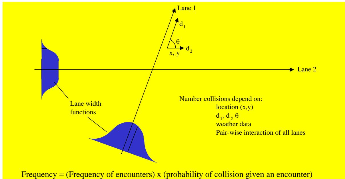
**Figure 13-4: Graphical representation of the collision model**
