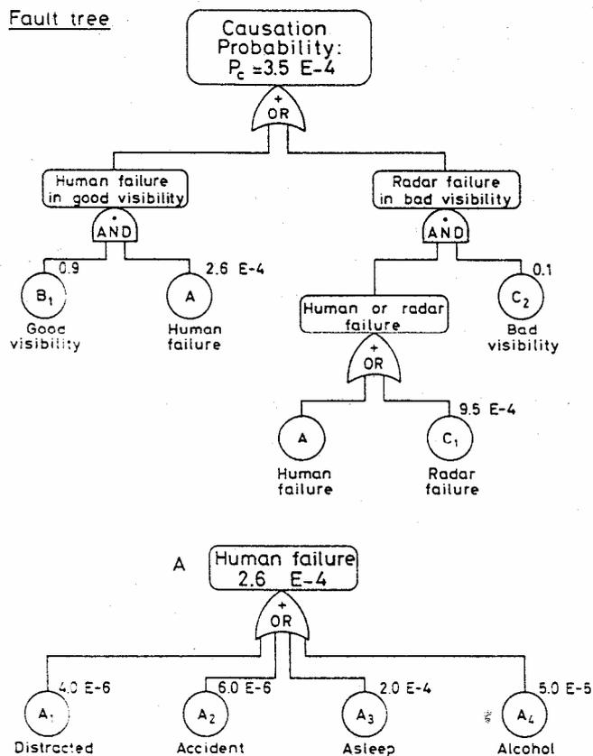
**Figure 7-1: Fault tree for causation (human failure) probability.**
