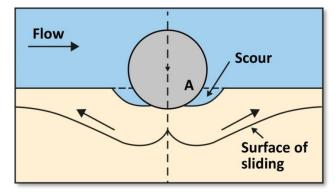
Figure 3.3 – Scour mechanism
