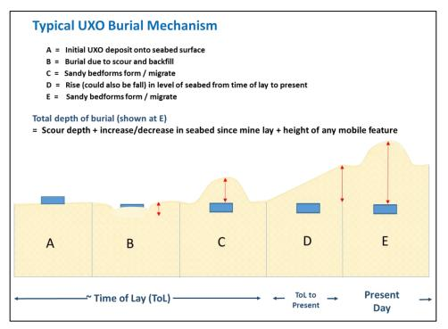
*Figure 3.2 – Typical UXO burial mechanisms*
