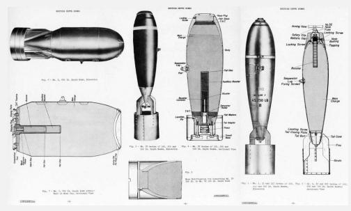
British Anti-Submarine Depth Bombs: L-R Mk I 600lb, Mk IV Series, Mk I-III Series
