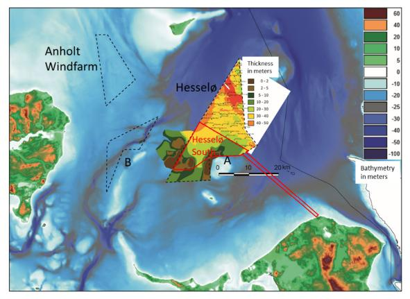
Figure 9.4 General thickness of geotechnical soft sediments (combined thickness of seismic Units A–E/F) in the current Hesselø South OWF area compared with the detailed mapping of the previous Hesselø OWF area. The Hesselø South OWF area and cable route is shown with red together with the existing Anholt OWF and OWF areas covered in previous screening reports (black hatched lines).
