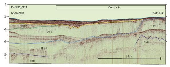
Figure 9.3 Northwest to southeast section through the Hesselø South OWF area. For location see Figure 9.1. The seismostratigraphic units are shown in Table 1.
