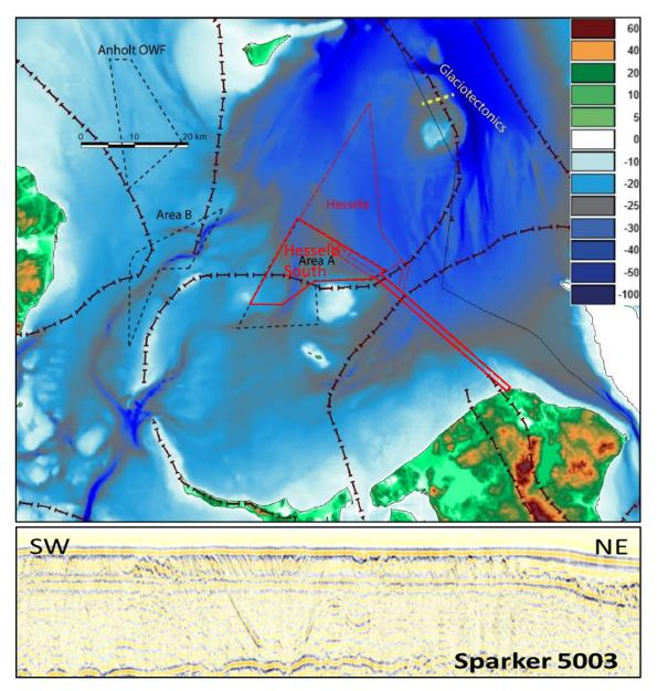
Figure 5.6. Upper figure: Interpreted ice marginal ridges in the southern part of the Kattegat. Lower figure: Sparker profiler showing evidence of glaciotectonic deformations north of Store Middelgrund (yellow dashed line on upper figure). The Hesselø South OWF area and cable route is shown with red together with the existing Anholt OWF and OWF areas covered in previous screening reports (black and red hatched lines). Bathymetry from www.emodnet-bathymetry.eu.
