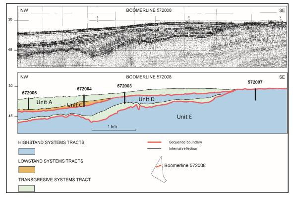
Figure 6.2. Boomer seismic section 572008.
