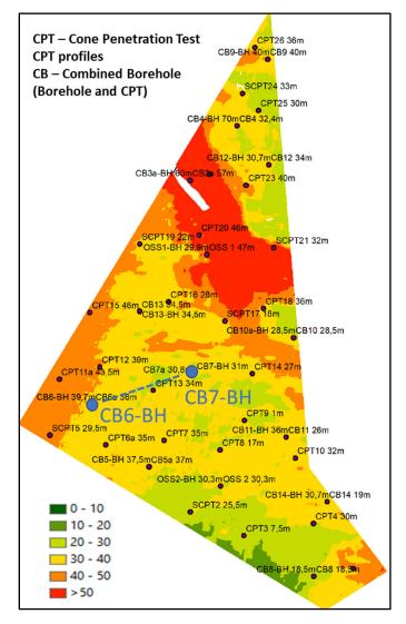
Figure 7.3 Thickness of geotechnical soft sediments (combined thickness of seismic Units A–E/F) in the previous Hesselø OWF area. Point data show thickness of soft sediments (CPT and boreholes). There is generally a good correlation between the data sets. Local areas without correlation could be related to glacial disturbance of Unit E/(F). Figure from Energinet (2021).
