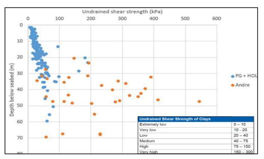
Figure 7.2 Undrained shear stress measurements showing low Unit A - E/F values and higher values for the lower units G–H.
