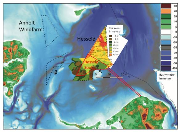
Figure 12.1 General thickness of geotechnical soft sediments (combined thickness of seismic Units A–E/F) in the current Hesselø South OWF area compared with the detailed mapping of the previous Hesselø OWF area. The Hesselø South OWF area and cable route is shown with red together with the existing Anholt OWF and OWF areas covered in previous screening reports (black hatched lines).
