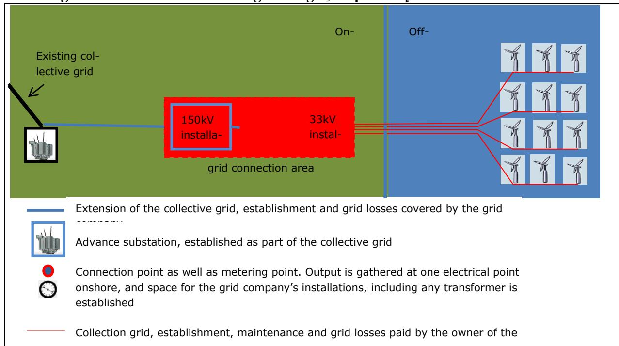
*Example for supply of total output of 33 kV, and where, because of grid losses in the collective grid, it is necessary to establish an advance 150/33 kV substation.*
