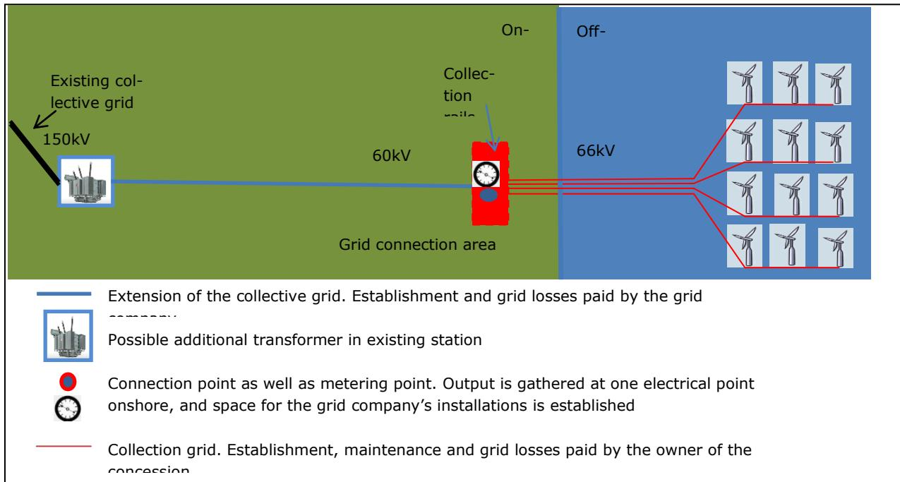
*Example for supply of total output of 60 kV, and where it is optimal in a socio-economic context to transport the output at 60kV onwards to an existing station.*
