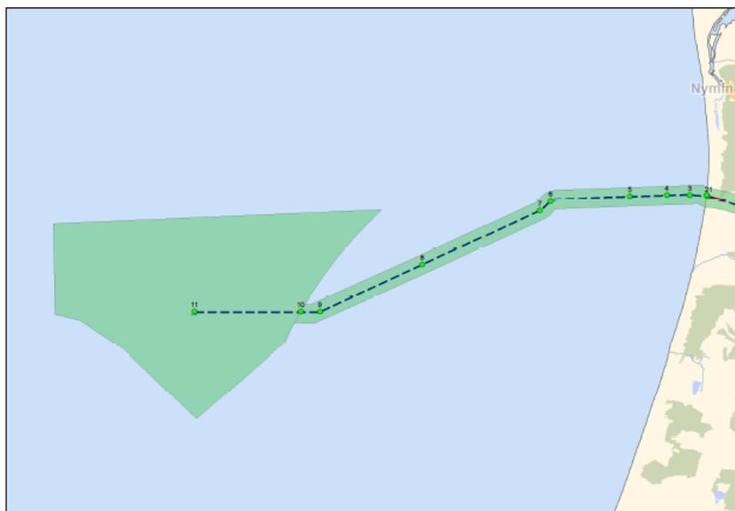
Figure 1. Location of the Horns Rev 3 OWF (400 MW) and the projected corridor for export cables towards shore. The area enclosed by the polygon is app. 160 km<sup>2</sup>.
