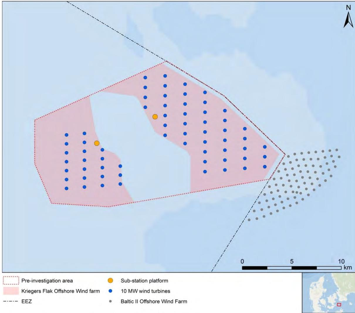
**Figure 2.3 Proposed layout for 10 MW turbines at the eastern and western part of the planned Kriegers Flak OWF.**
