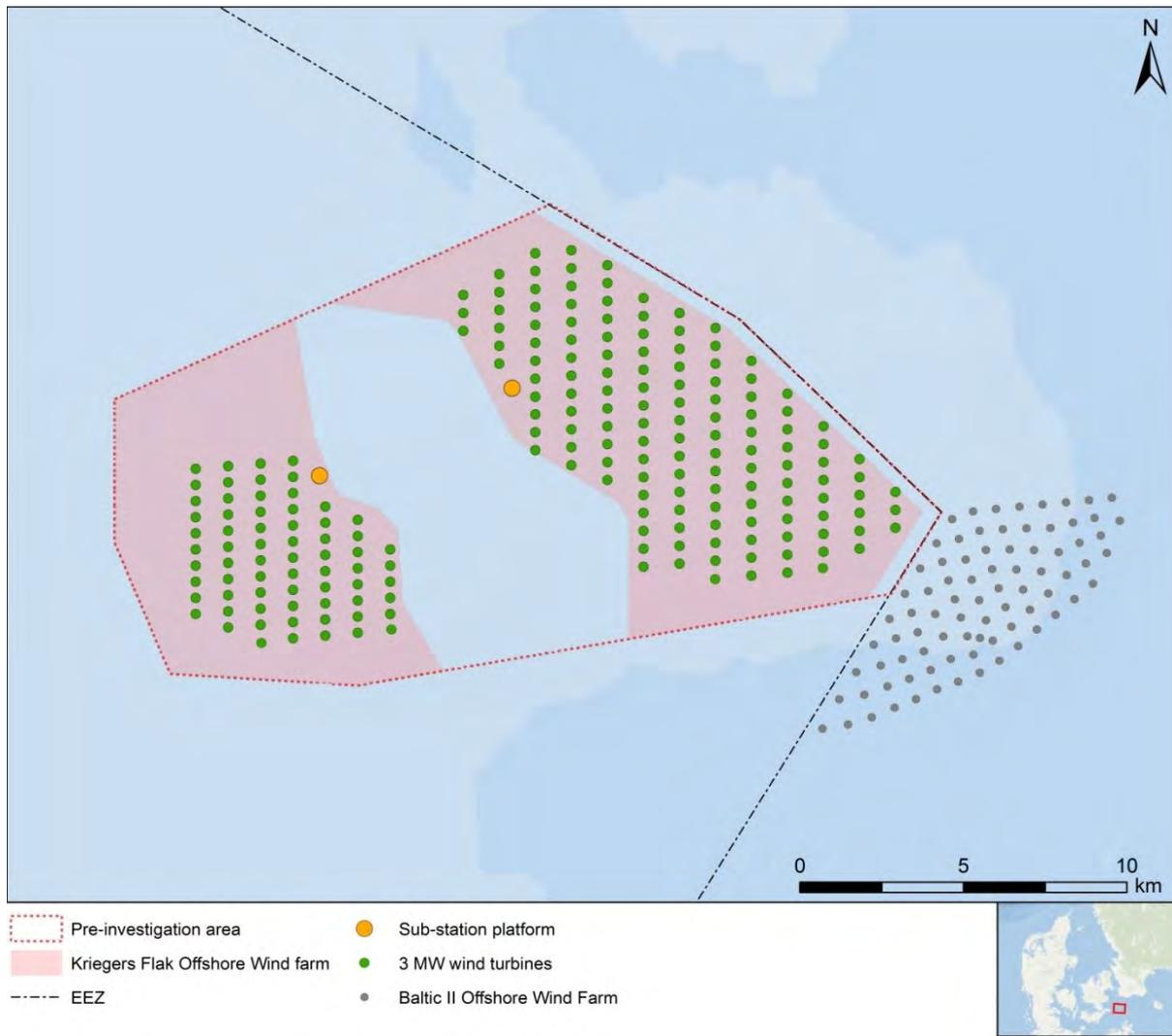
**Figure 2.2** Proposed layout for 3 MW turbines at the eastern and western part of the planned Kriegers Flak OWF.
