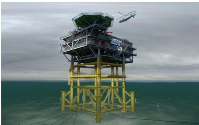
**Figure 3-6** Substation installed with a jacket foundation.
