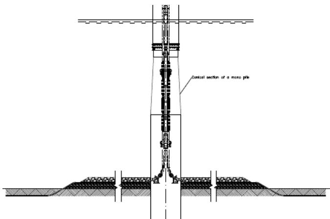
**Figure 3-4 Schematic illustration of a driven steel monopile.**
