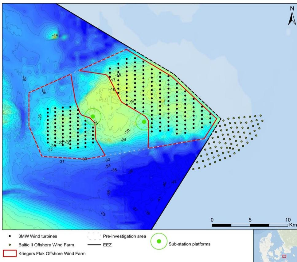
Figure 3-2 Layout of 203 wind turbines on Kriegers Flak using 3 MW turbines only.
