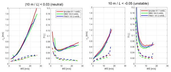
Figure C-2: Mean (full line) and standard deviation (dashed line) of  $\sigma_U$  and TI measured at three different offshore met masts, for neutral (left) and unstable (right) conditions.
