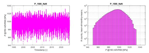
Figure 6-14: The left part of the figure shows the modelled time series of air pressure at 150 mDVR90 from the Vortex mesoscale dataset at the NSI-LB-3 location. The right part of the figure shows an MoMM histogram of the modelled values with a logarithmic 2<sup>nd</sup> axis.
