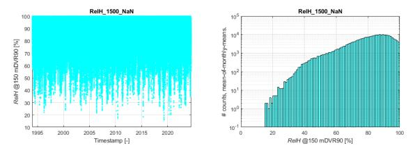
Figure 6-12: The left part of the figure shows the time series of the hourly mean values of relative humidity at 150 mDVR90 from the Vortex mesoscale dataset at the NSI-LB-3 location. The figure on the right shows an MoMM histogram of the modelled values with logarithmic  $2^{nd}$  axis.
