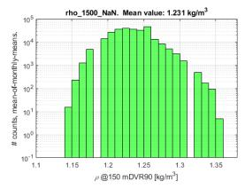
Figure 6-15: Air density at 150 mDVR90 from the Vortex time series computed at the NSI-LB-3 location. The left part of the figure shows the model time series, and the right part of the figure shows an MoMM histogram of the model values with a logarithmic  $2^{nd}$  axis. The MoMM mean value is shown in the title above the histogram.
