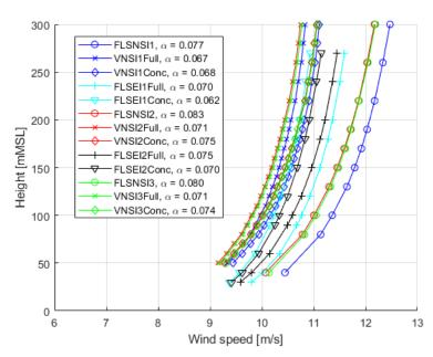
Figure 6-2: Mean wind speed profiles and fitted shear exponents to the 3 NSI FLSs, their co-located Vortex model time series, and the 2 EINS FLSs.
