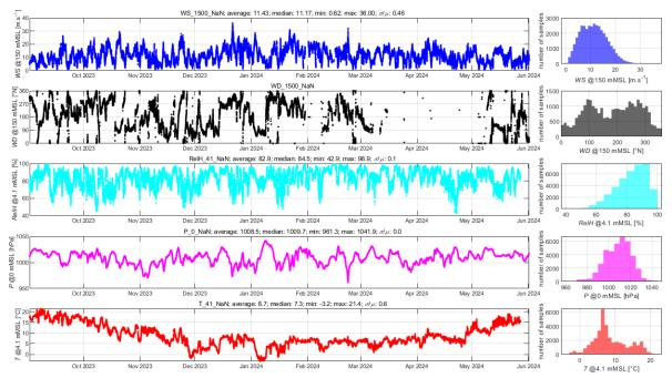
Figure B-3: Time series of wind speed and wind direction at 150 mMSL, as well as surface level air temperature, relative humidity and air pressure collected at NSI-2-LB.
