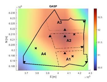
Figure 5-4: Spatial variation of 10-minute wind speed with a 50-year return period at 150 mMSL, from the GASP dataset. The coloured background follows the colour scale on the right. The highest value found within each sub-area is marked with an upwards-pointing triangle, the lowest value with a downwards-pointing triangle, and the locations of the 3 FLSs as crosses. CRS: WGS84 / UTM Zone 32N.
