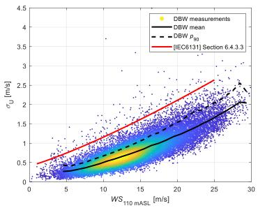
Figure C-4: This figure shows measured turbulence intensity values in neutral conditions at the DBW met mast (scatter, full and dashed black lines), and the 90<sup>th</sup> percent quantile modelled using the guidance in [IEC6131] (red line).
