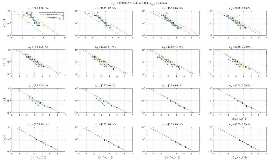
Figure C-6: Same as Figure C-5, with two additional stability classes: near-neutral stable (light blue), and stable (blue). The model overprediction of measured values for stable classes has been addressed as described in the text.
