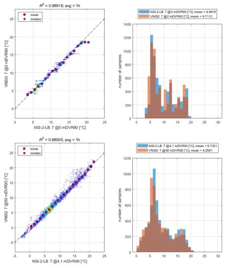
Figure 6-8: Scatter plots and histograms between temperatures measured by NSI-LB-2 and from the colocated Vortex model. **Top**: sea surface temperature for both datasets; **bottom**: air temperature measured at 4.1 mSWL and modelled at 50 mMSL.
