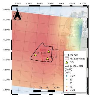
Figure 8-6: Reproduction from [GASP] of map of 50-year 10-minute mean extreme wind speed estimates at 150 m (assumed to be 150 mDVR90 – see the text above). CRS: WGS84.
