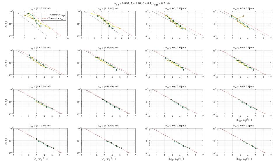
Figure C-5: For unstable (yellow), near-neutral unstable (brown) and neutral (green) stability conditions, and for several bins of surface friction velocity, this figure shows measured mean ratios  $(\sigma_U(z)/u_{*0})^2$  as a function of  $z/z_i$ . The black line shows the original Townsend model (Eq. C-6), the red line shows the modified model (Eq. C-7).
