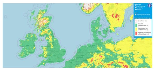
Figure 9-2: IEA wind turbine icing classes, from <a href="http://virtual.vtt.fi/virtual/wiceatla/">http://virtual.vtt.fi/virtual/wiceatla/</a>.
