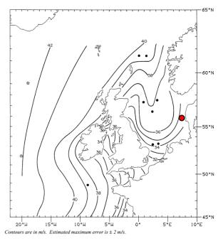
Figure 8-3: Contours of 50-year 1-hour mean 10 mMSL wind speed over Northern Europe, from Figure 1 of [UKHSE]. According to Section 3.3b) of ibid., the values can be converted to 10-minute mean values at 10 mMSL as described in the text, and using Section 3.3c) of ibid., the value can be extrapolated to 140 mMSL, and further extrapolated to 150 mDVR90 using the shear exponent in Section 8.1. The location of the project site is shown with a red circle. CRS: WGS84.
