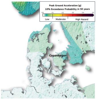
Figure 9-1: Map and colour bar showing the 475-year return period PGA, extracted from the [SHARE] database. Note that the values are in units of g, yielding a PGA interval at the site of <0.25-0.29 m/s<sup>2</sup>.
