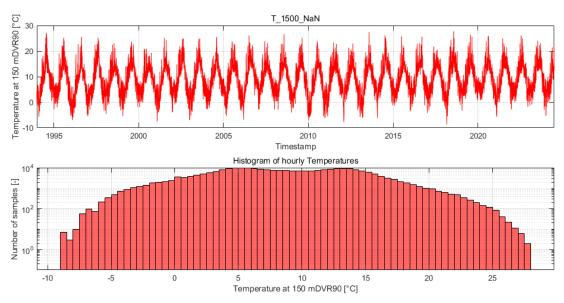
Figure 6-9: Top: time series of hourly air temperature at 150 mDVR90 from the Vortex dataset at the NSI-LB-3 location. Bottom: Histogram, with a logarithmic  $2^{nd}$  axis, corresponding to the time series in the top part of the figure.
