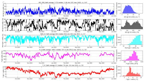
Figure B-2: Time series of wind speed and wind direction at 150 mMSL, as well as surface level air temperature, relative humidity and air pressure collected at NSI-1-LB.
