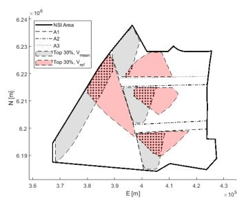
Figure 5-5: NSI area and subdivisions with the locations of the highest 30% mean wind speed (grey) and extreme wind speed (red). The representative analysis points for each subdivision are defined from the intersection of both areas. CRS: WGS84 / UTM Zone 32N.
