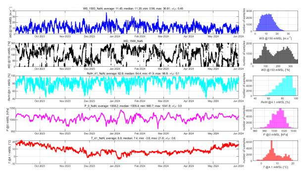
Figure B-4: Time series of wind speed and wind direction at 150 mMSL, as well as surface level air temperature, relative humidity and air pressure collected at NSI-3-LB.
