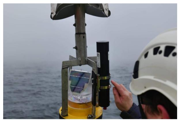
Figure 2 - Automatic bat detector mounted on a PAM-buoy for the marine mammal survey.
