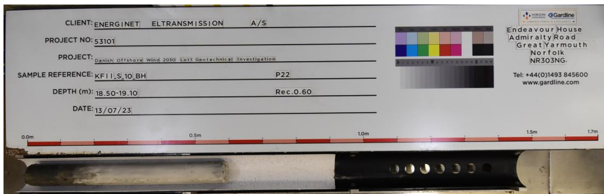
Figure 6-25 - KFII_S_10_BH example of till to chalk interface
