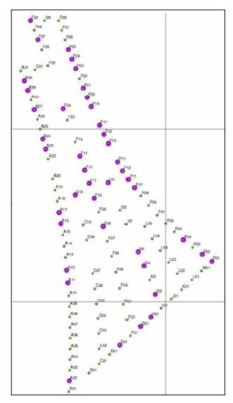
Figure 2: Layout and position of turbines in Anholt Offshore Windfarm. Positions coloured in purple indicate the WTG positions with scour protection.
