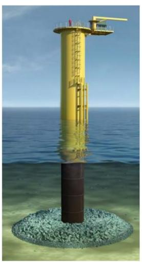
Figure 3: Typical monopile foundation with scour protection pad.
