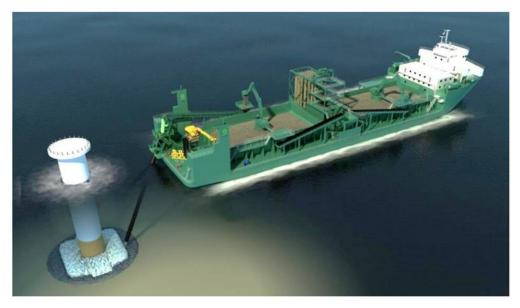
Figure 10: Example inclined fall pipe rock installation vessel showing the at deployment of the fall pipe next to a monopile.
