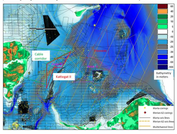
Figure 4.1. Distribution of Marta database seismic grid and core data in the southern and central Kattegat region. The Kattegat II OWF area and cable corridor is shown in red and green together with the existing Anholt OWF and OWF areas covered in previous screening reports (purple and red hatched lines). Bathymetry from <a href="https://www.emodnet-bathymetry.eu">www.emodnet-bathymetry.eu</a>.
