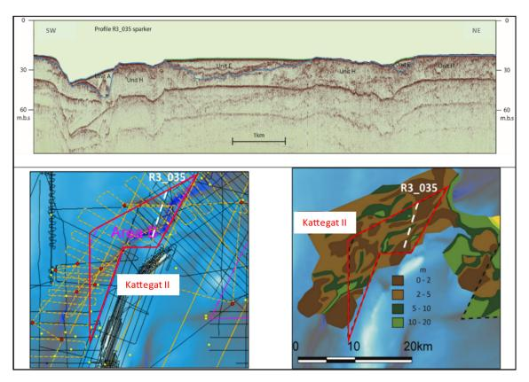
Figure 9.1 Southwest to northeast Sparker profile R3\_035 with location in relation to the seismic archive data grid (black lines are Sparker data) and the geotechnical soft sediment thickness map.
