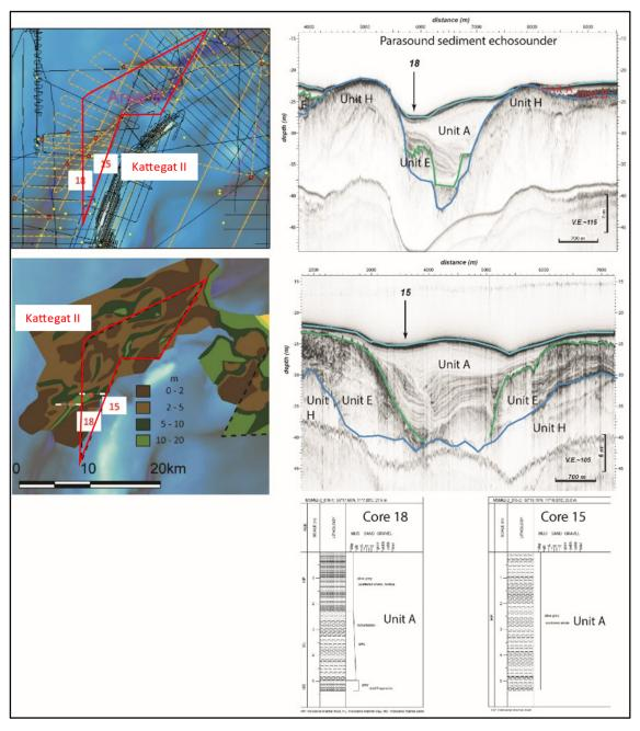
Figure 9.5 Parasound echosounder profiles from the southern part of the Kattegat II OWF area, with location in relation to the seismic archive data grid (yellow lines are Parasound data). The positions of the seismic profiles and vibrocores 18 and 15 are indicated on the geotechnical soft sediment thickness map. Core descriptions with indication of seismic units are shown below the seismic profiles.
