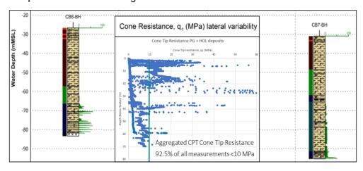
Figure 7.1 Geotechnical sediment cores CB6-BH and CB7-BH, with indication of very low cone resistance to more than 40 m below seabed and evidence of 92,5% of total CPT measurements below 10 MPa. The location of CB6-BH and CB7-BH is indicated on Figure 7.3.
