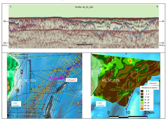
Figure 9.6 South to north Sparker profile AS\_SC\_02b with location in relation to the Sparker seismic archive data (black lines are archive Sparker data, yellow lines Parasound data and purple lines are new Sparker data) and the geotechnical soft sediment thickness map.
