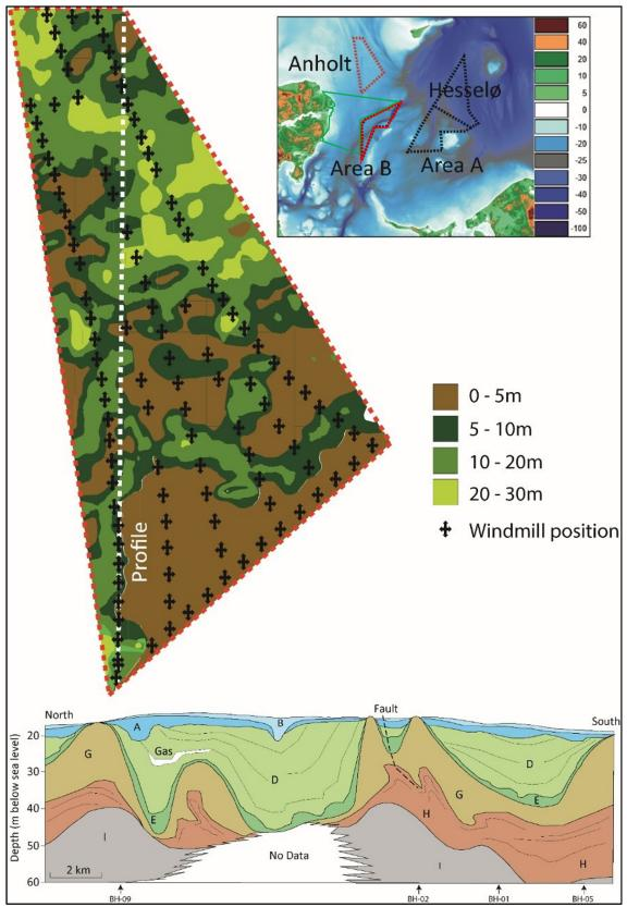
Figure 10.1 Anholt OWF general map of thickness of geotechnical soft sediment, with indication of location of schematic profile and windmill positions. Details of seismic units A–I in the schematic profile are provided in Table 1.
