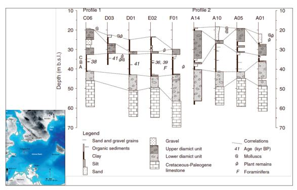
Figure 5.4. Cross-section of the deep cores at Kriegers Flak OWF showing the top of the Pre-Quaternary varying between c. 40 and 55 m b.s.l. From Anjar et al. (2010).
