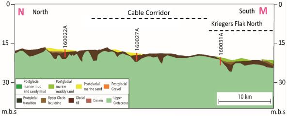
Figure 8.3 Upper figure: Surface sediments in the outer Faxe Bay region. Location of Baltic Pipe profile profile N - M is indicated. Lower figure: Interpretation of Baltic Pipe seismic profile N - M with indication of Kriegers Flak II North.
