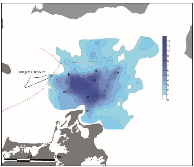
Figure 6.7 Thickness of Holocene mud by Lemke (1998). Location of Kriegers Flak II South OWF is shown with black dashed lines. The red dashed lines show the EEZ.
