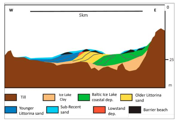
Figure 6.3. A simplified geological model of the Kriegers Flak OWF showing the different stages of coastal, sandy progradation. From Jensen 2019.
