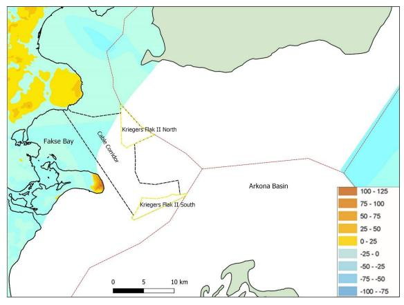
Figure 5.3 Pre-Quaternary surface topography in metres above sea level (Binzer & Stockmarr 1994). Location of Kriegers Flak II North and Kriegers Flak II South and the cable corridor is shown with dashed lines. The red dashed lines show the EEZ.
