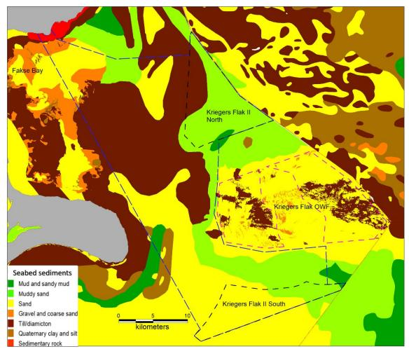
Figure 7.2. Seabed sediment map around the Kriegers Flak II North and South (black dashed lines) and cable corridor (blue dashed lines) areas. The map is based on a combination of the EMODnet 1:1M seabed substrate map and the Danish 1:100.000 (2020 version) seabed sediment map. The existing Kriegers Flak OWF (purple dashed lines) and the EEZ (red dashed lines) are indicated.
