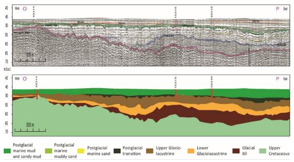
Figure 8.6 Baltic Pipe sparker profile O - P (upper figure) and geological interpretation (lower figure). Vibrocore positions are marked with red lines. For location, see figure 8.4.
