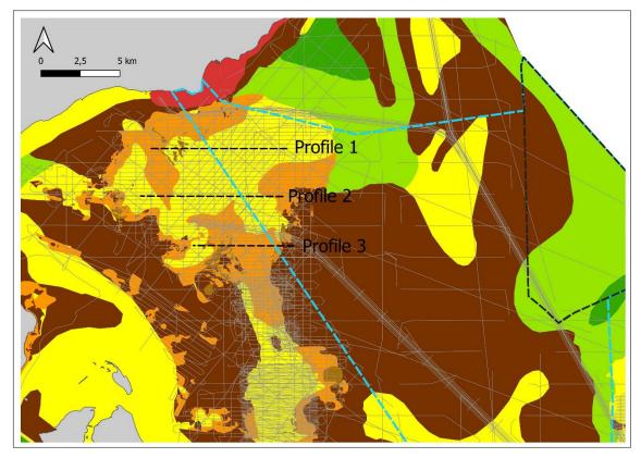
Figure 8.15 Map showing the location of three seismic profiles (black hatched lines) illustrating the stratigraphy in the Faxe Bay and the northern part of the cable corridor (blue hatches lines).
