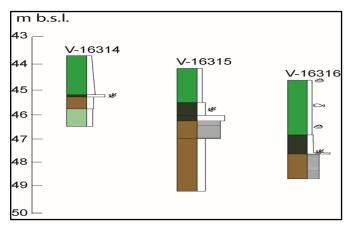
Figure 8.5 Vibrocore logs along Baltic Pipe profile O – P. See Figure 8.6 for legend.
