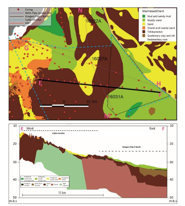
Figure 8.1 Upper figure: Surface sediments in the outer Faxe Bay region with the location of Baltic Pipe profile E - F indicated. Lower figure: Interpretation of Baltic Pipe seismic profile E - F with indication of the Kriegers Flak II North.
