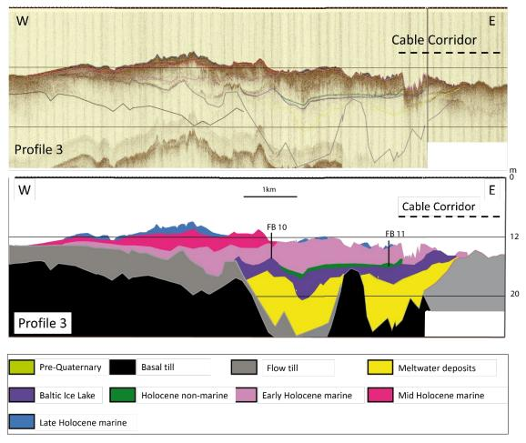
Figure 8.16. Interpreted seismic profiles from the outer part of Faxe Bay. The crossing of the cable corridor is marked with the hatched lines. Redrawn from Lomholt et al. 2016.
