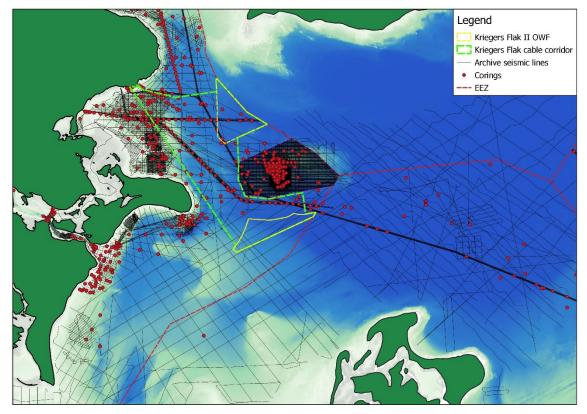
Figure 4.1. Overview of data in the study area and the adjacent area. The Kriegers Flak II North and South are indicated by yellow dashed lines; the cable corridor by light green dashed lines. The EEZ shown by red dashed lines. The background bathymetry map is from Emodnet <u>www.emodnet-bathymetry.eu.</u>
