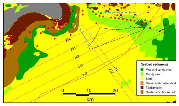
Figure 8.4 The seismic lines described in the text (pink dashed lines) and vibrocores (red dots) on top of the seabed sediment map. Kriegers Flak II South OWF marked with dashed black lines, the cable corridor with blue lines, and the EEZ with red dashed lines.
