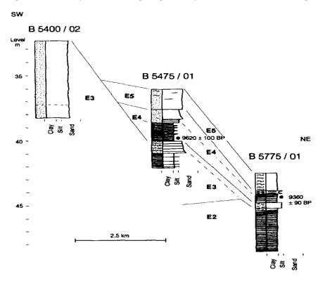
Figure 8.10 Vibrocore logs along Boomer profile 242, from Jensen et al. (1997).
