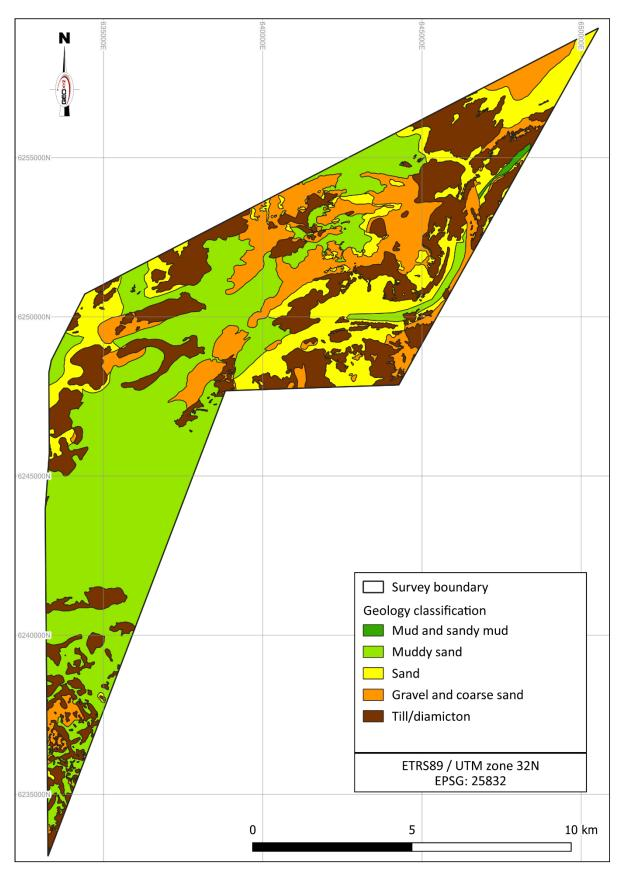
Figure 39: Seabed surface geology classification
