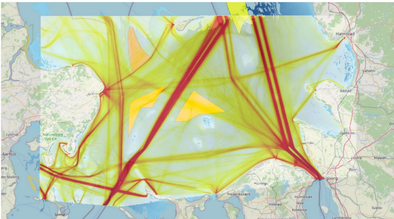
Figure 5-2 Vessel routes based on AIS data from 2022. The offshore wind farm areas Kattegat and Hesselø are shown as orange. Kattegat is located west and Hesselø east. Source: HAZID Report Kattegat (DNV, 2024)
