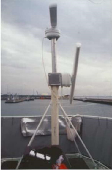
Figure 4-4 Horizontal and vertical radar mounted on a research vessel.
